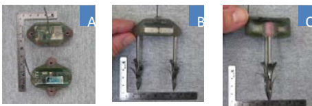
Fig. 1. Original location-only SPOT5 LIMPET tag (A [top] and B) and new Mk10-A depth-transmitting LIMPET tag (A [bottom] and C). Tags attach with 2 titanium barbed darts that penetrate 6.5 cm.
